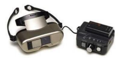
Similar in function to the visor worn by the blind character Geordi LaFarge in Star Trek: The Next Generation, the JORDY<sup>TM</sup> (Joint Optical Reflective Display by medical device manufacturer Enhanced Vision of Huntington Beach, CA) magnifies objects up to 50 times and allows changes in contrast, brightness, and display modes.
